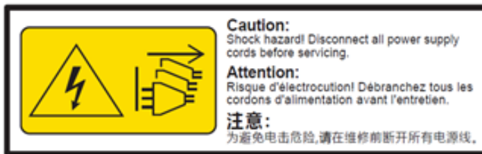
Figure 8-2 Multi-power Safety Protection
